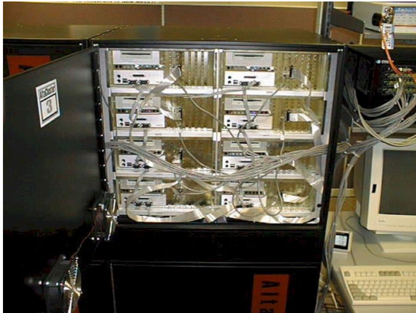
Figure 6. Inside a Roadrunner cabinet with each node attached to three networks: Myrinet (ribbon cable), Fast Ethernet (CAT5), and Diagnostic (RS232 serial port). (Image credit: Courtesy of the author.)
