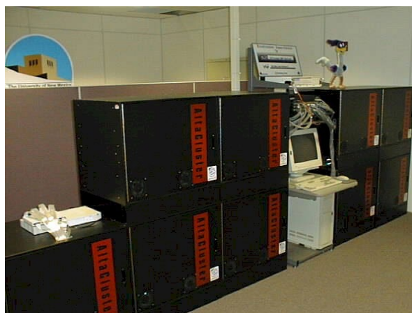
Figure 4. Linux prototype on lower-left, and Roadrunner (right). A Myricom dual 8-port SAN Myrinet switch sits on top of the left-most cabinet of the prototype, and four octal 8-port SAN Myrinet switches (not visible) connect Roadrunner. Above Roadrunner's console is a 72-port Foundry Fast Ethernet switch with Gigabit uplinks to the vBNS and Internet. (Image credit: Courtesy of the author.)
