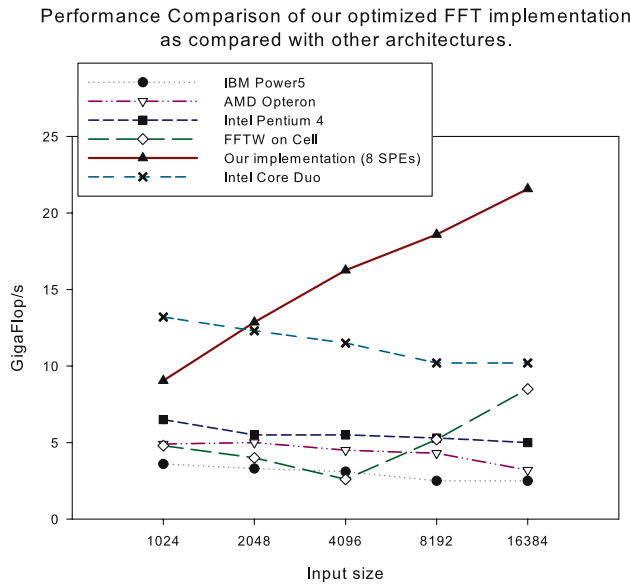
Fig. 7. Performance comparison of FFTC with other architectures for various input sizes of FFT. The performance numbers are from benchFFT from the FFTW website.
