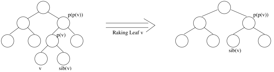
Fig. 2. Rake of leaf v : removes vertices v and p(v) from the tree and makes the sibling sib(v) of vertex v , the child of grandparent p(p(v)) of v
