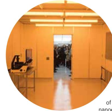
NJIT's recently opened **Microfabrication Innovation Center** houses equipment and a cleanroom environment for the fabrication of microelectronic, nanoelectronic and microfluidic devices and sensors. Its rooms are free of potentially contaminating particles larger than a micron; the highest-level cleanroom is limited to 100 1-micron particles in a cubic meter of air.
