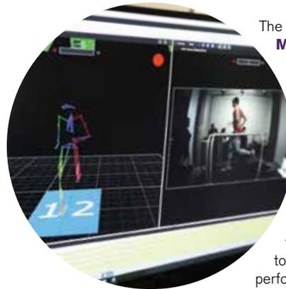
The **Life Sciences Motion Capture Lab** decodes the complexities of human movement using infrared cameras, an instrumented treadmill, electromyography and inertial sensors. This technology is used to study human performance, sports injuries, musculoskeletal disorders and the use of assistive devices, such as robotic exoskeletons, to improve human movement.
