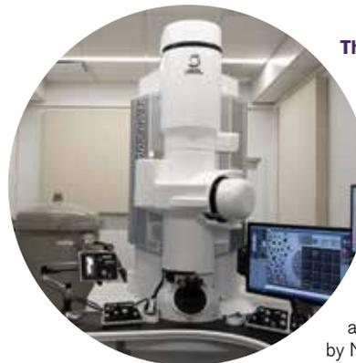
The **transmission electron microscope (TEM)** sends a beam of electrons through objects to capture fine details of structures as tiny as atoms. Used by NJIT chemists, pharmaceutical engineers, materials scientists and others, the TEM elucidates structures of crystals, for example, which can be manipulated to alter material properties.
