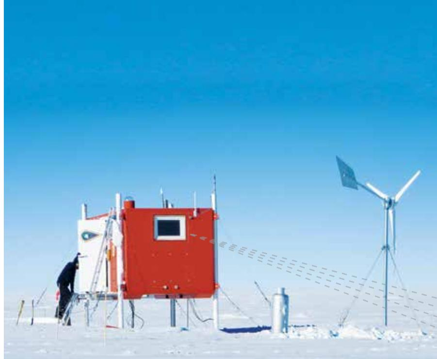
NJIT's automatic geophysical observatories in Antarctica's frozen wilderness house instruments that measure fluctuations in the magnetic lines caused by solar wind and light from the Aurora Australis, the luminous collision of charged particles drawn by the South Pole's magnetic field. They provide continuous data sets of the larger geospace environment, which cannot be captured from instruments orbiting in space.
