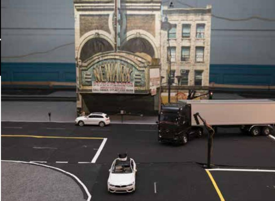
Photo right: (left to right) Carlos Maranon, Zarin Rahman, Nishaant Goswamy and Alexis Brice developed automotive systems for a fleet of toy vehicles (photo left) that will drive on the streets of a miniaturized Newark, N.J., in an experiment designed to evaluate the impacts of connected and automated vehicles on drivers, passengers in autonomous cars and pedestrians.
