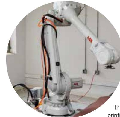
The **seven-axis robot arm, IRB 4600**, performs tasks ranging from picking-and-placing, milling, drawing and even three-dimensional printing. Architecture and design students are building attachments, or effectors, for the arm that have it sorting bricks by color and then stacking them accordingly with a pneumatic gripper.
