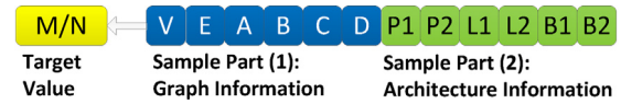
Fig. 10. Each training sample contains the graph and the architecture information. V and E are the number of vertices and edges respectively. A , B , C , D are the parameters used in graph construction (Table 1). P1 , L1 , and B1 are the peak performance, L1 cache size, and memory bandwidth, respectively, of the platform that top-down method runs on. P2 , L2 , B2 are those of the platform that bottom-up method runs on.
