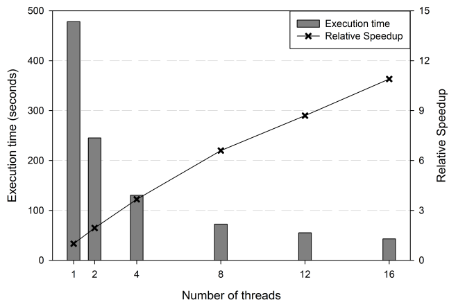
Figure 10. Parallel BFS performance on the IBM Power 570 system for an R-MAT graph of 500 million vertices and 4 billion edges.
