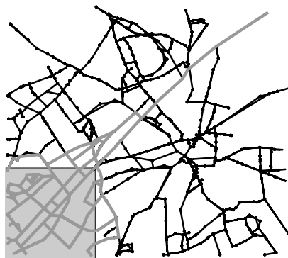
FIGURE 2. The search space of an arc-flag-accelerated Dijkstra search: the search started in s and the region containing the target node t is highlighted.
