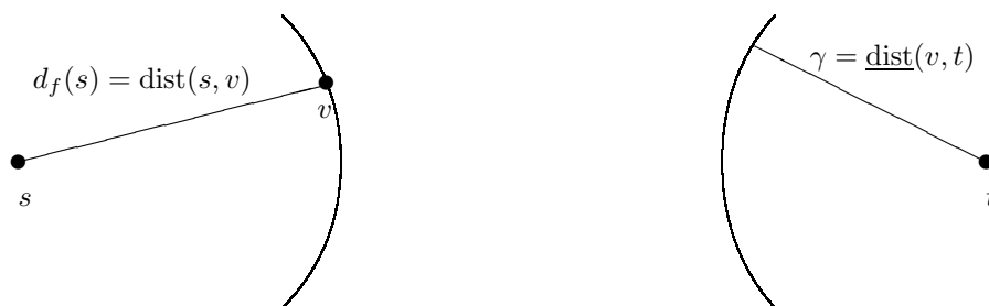
FIGURE 2. Pruning using implicit bounds. Assume v is about to be scanned in the forward direction, has not yet been scanned in the reverse direction, and that the smallest distance label of a vertex not yet scanned in the reverse direction is \gamma . Then v can be pruned if \bar{r}(v) < d_f(v) and \bar{r}(v) < \gamma .
