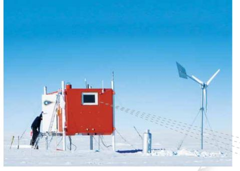
NJIT's automatic geophysical observatories in Antarctica's frozen wilderness house instruments that measure fluctuations in the magnetic lines caused by solar wind and light from the Aurora Australis, the luminous collision of charged particles drawn by the South Pole's magnetic field. They provide continuous data sets of the larger geospace environment, which cannot be captured from instruments orbiting in space
