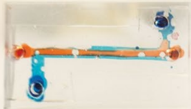
With an NIH grant, Lowe-Krentz, Liu and Ou-Yang are learning to grow human endothelial cells on channels patterned into a finger-sized chip.
